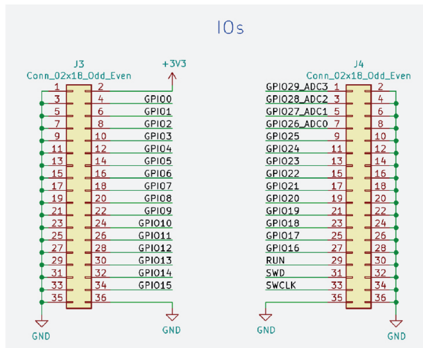
Figure 10. Schematic section showing the 2.54mm IO headers
